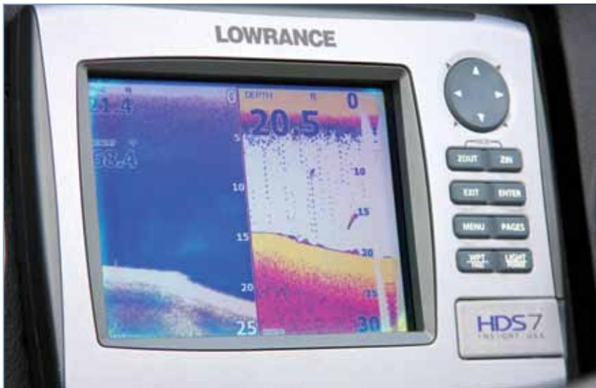
*This depth finder offers the ability to show water depth, suspended fish and water temperature. It also has an integrated GPS and mapping capability. On unfamiliar waters, this type of unit will both find fish and help you boat safely.*
