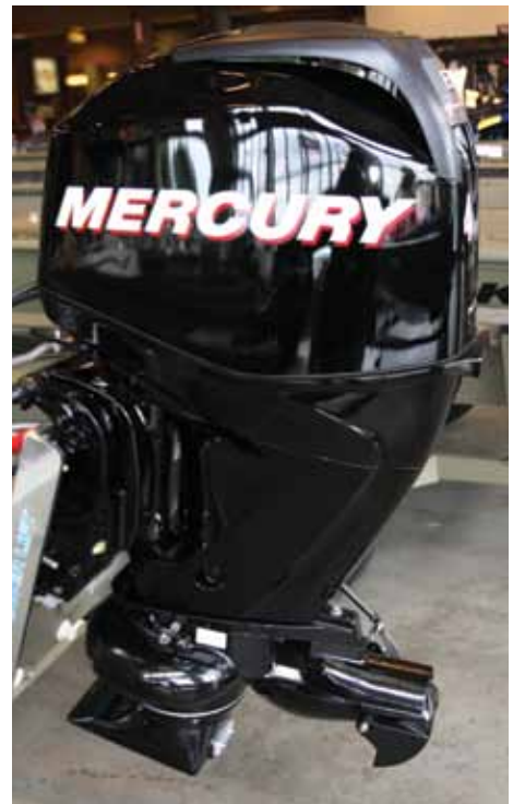
A jet drive motor is useful in many shallow rivers like the Susquehanna, Delaware, Juniata and more. Keep your aluminum bass boat fishing and problem free in rocky situations with a jet.
