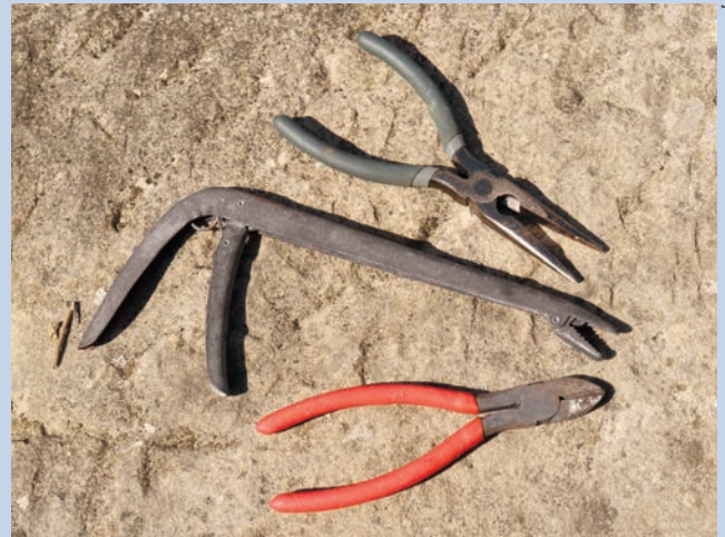
Tools for unhooking fish (from top to bottom): long nose pliers, hook removal tool and diagonal wire cutters for cutting bait hooks that cannot be removed without harming the fish.
