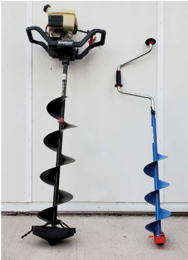
Ice augers are the most important part of your ice fishing setup. Ice augers come in both powered and hand-driven models. Some newer ice augers attach to cordless drills or may be powered by lithium batteries.
