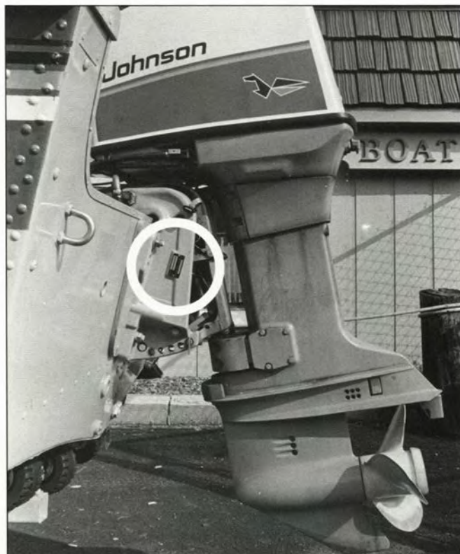
The model number and serial number of an engine appear on a plate (circle) that's located on the motor's clamping bracket or on the swivel bracket. Some manufacturers place this information inside the cowling, so look there if you can't find the numbers on the outside of the motor.
