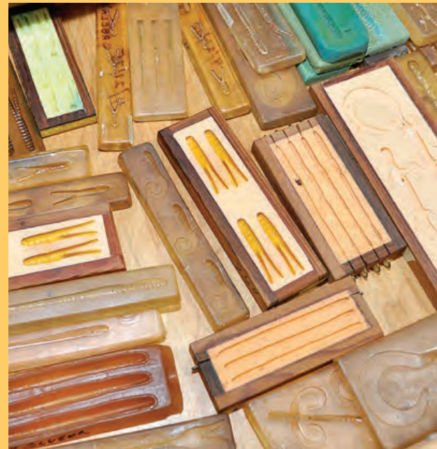
Acrylic single pour molds, many dating to the 1970s, are sometimes used to fulfill a custom order for a customer.
