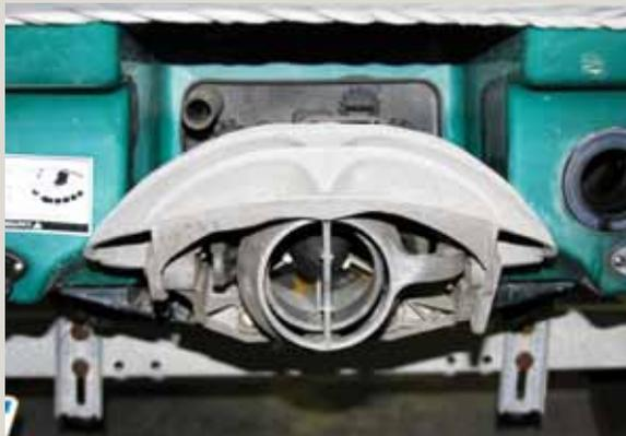
*Inspect the discharge area of your PWC for damage from rocks and other items, and keep it in good working order. If you operate your PWC in saltwater, it should be flushed regularly in-season, in addition to flushing before storage.*
