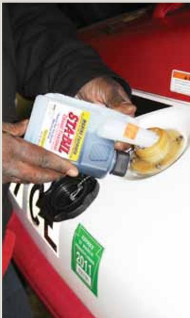
*Add a fuel stabilizer to the gas tank of your PWC, and run it for a short period of time to prevent build-up from evaporating gasoline during storage.*
