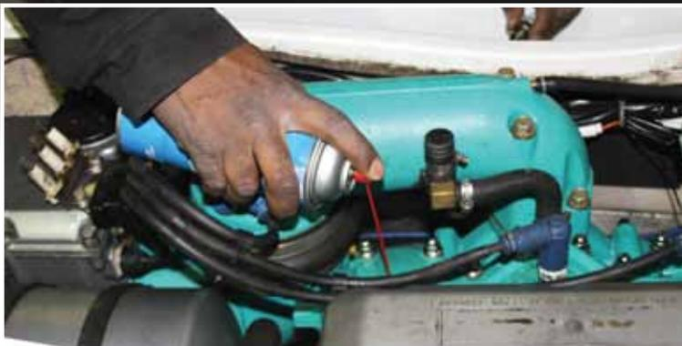
*(Above) Use fogging oil to help prevent engine rust and corrosion during storage of your two-stroke PWC. This photo shows applying the oil into a cylinder of a two-stroke PWC after removing the spark plug.*
