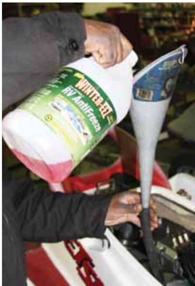
*(Right) Recreational vehicle antifreeze should be ran through your PWC before storage for the winter to ensure that there are no cracked or leaking parts due to freezing and thawing water. Make sure to appropriately dispose of antifreeze and any other chemicals that you use when maintaining your PWC.*
