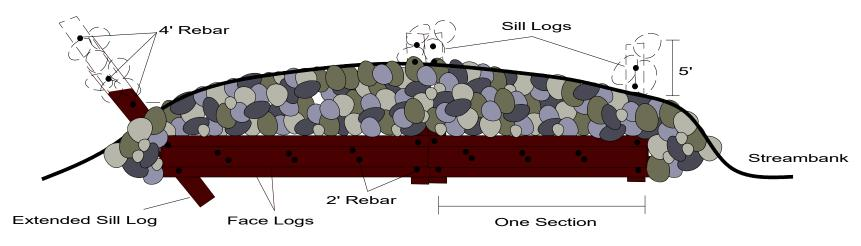
Note: Each section includes two sill logs and at least two face logs, sections can be added or removed
