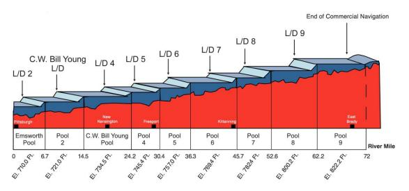
**Figure 5.12.** Generalized profile of locks and dams on the lower Allegheny River, depicting navigation pool elevations and upstream distances from Pittsburgh (modified from USACE 2010).
