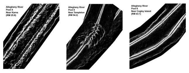
**Figure 6.2.** Side-scan sonar images of extensively dredged reaches of Allegheny River Pool 4 (left); Allegheny River Pool 8 dredge pit with scoop marks from clamshell dredge (center); and for comparison, an undredged reach of Allegheny River Pool 6 (right) (sonar images from USACE 2006).
