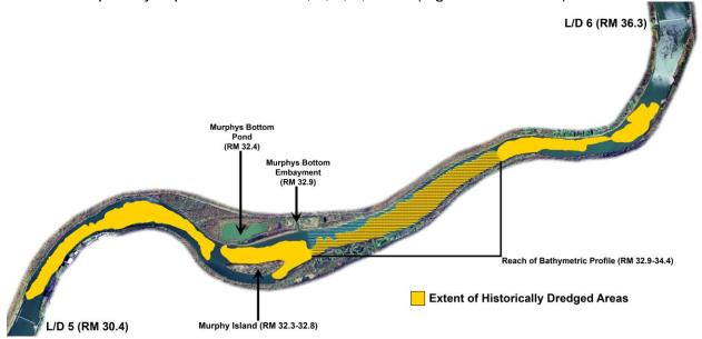
**Figure 6.1.** Dredged Allegheny River Pool 5. Yellow polygons depict historically dredged areas. Crosshatched area delineates river reach of the bathymetric profile shown in Figure 6.3 (photograph from PASDA 2010; dredged areas from USACE 2006).
