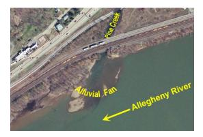
**Figure 7.4.** Confluence of Pine Creek and Allegheny River (RM 4.7) in Allegheny County. Pine Creek contributes a great deal of alluvial bedload to the Allegheny, most likely a result of Earth disturbance activities, impervious surfaces, and flashy hydrology of the contributing Pine Creek watershed, which drains several rapidly-developing northern suburbs of Pittsburgh. Arrow depicts direction of flow (modified aerial photograph from PASDA 2010).
