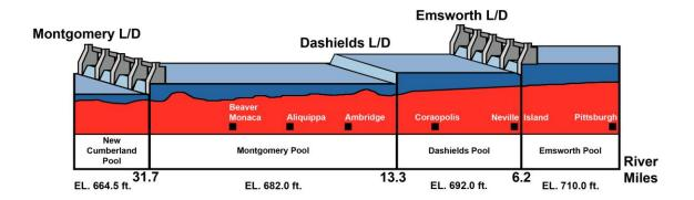
**Figure 5.11.** Generalized profile of locks and dams on the upper Ohio River, depicting navigation pool elevations and downstream distances from Pittsburgh (modified from USACE 2010).
