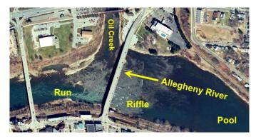
**Figure 7.1.** Pool-riffle-run sequence at confluence of Oil Creek and Allegheny River, Venango County (RM 131.9). This reach of river has historically maintained a riffle-run, tagged "Oil City Rapids" (Class II) by local whitewater enthusiasts. Arrow depicts direction of flow (modified aerial photograph from PASDA 2010).
