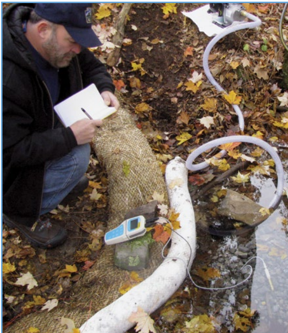
Pennsylvania Fish & Boat Commission (PFBC) Fisheries Biologist Steve Kepler (retired) taking water quality measurements in a stream with a handheld multiparameter meter.
