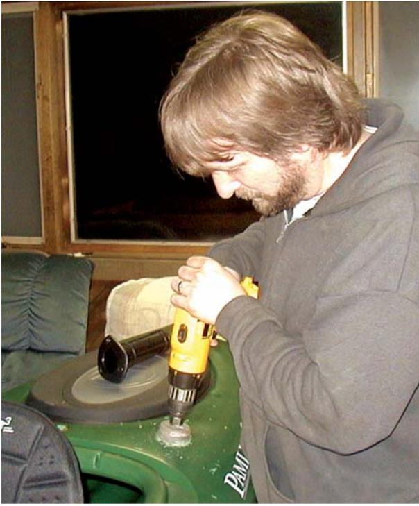
*After marking the location for a recessed rod holder, use the hole saw to cut the rough opening. Take time to measure twice and cut once: It just doesn't feel natural cutting a large hole into a perfectly good kayak!*
