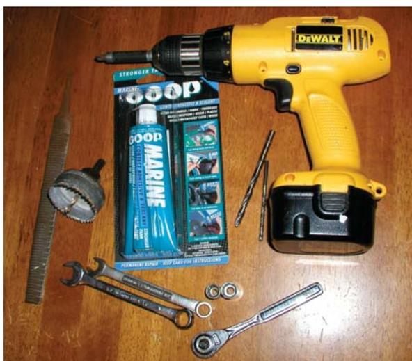
Basic tools you need include a Phillips-head screwdriver, drill, drill bits, a 3/8-inch and 7/16-inch wrench or socket set, and a rounded rasp file. If your plans involve any recessed accessories, you also need the correctly sized hole saw bit. Use a combination marine adhesive and sealant.
