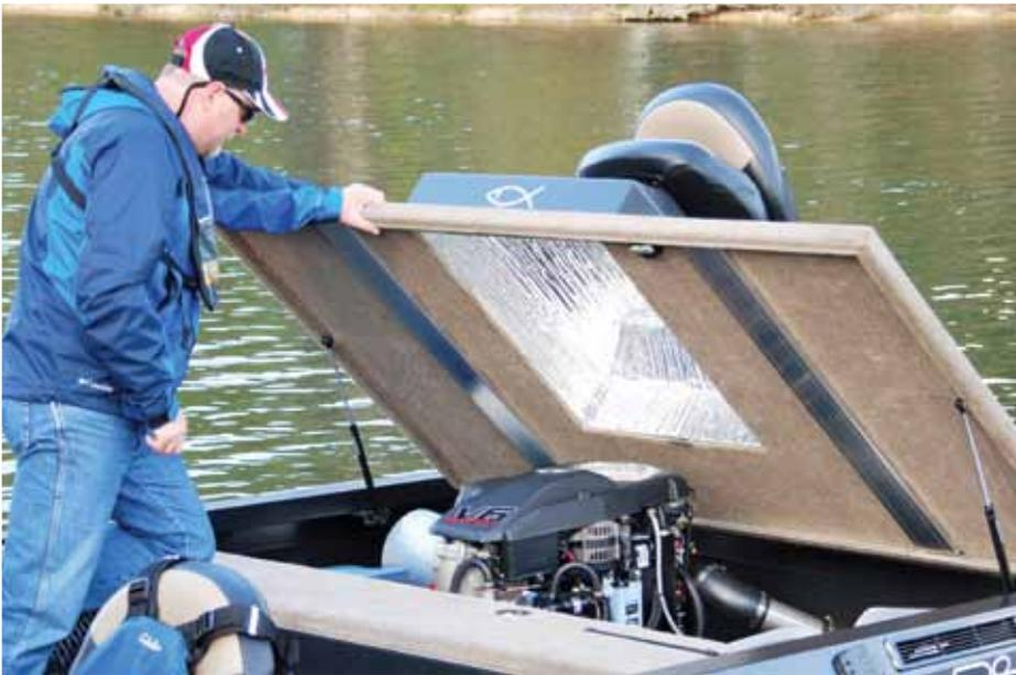
*With an inboard jet drive, the water enters the intake and after a short 28-degree ramp passes directly through the impeller and out the exhaust housing. The inboard jet pump does not have to redirect the water, giving it a significant performance edge to an outboard jet drive.*
