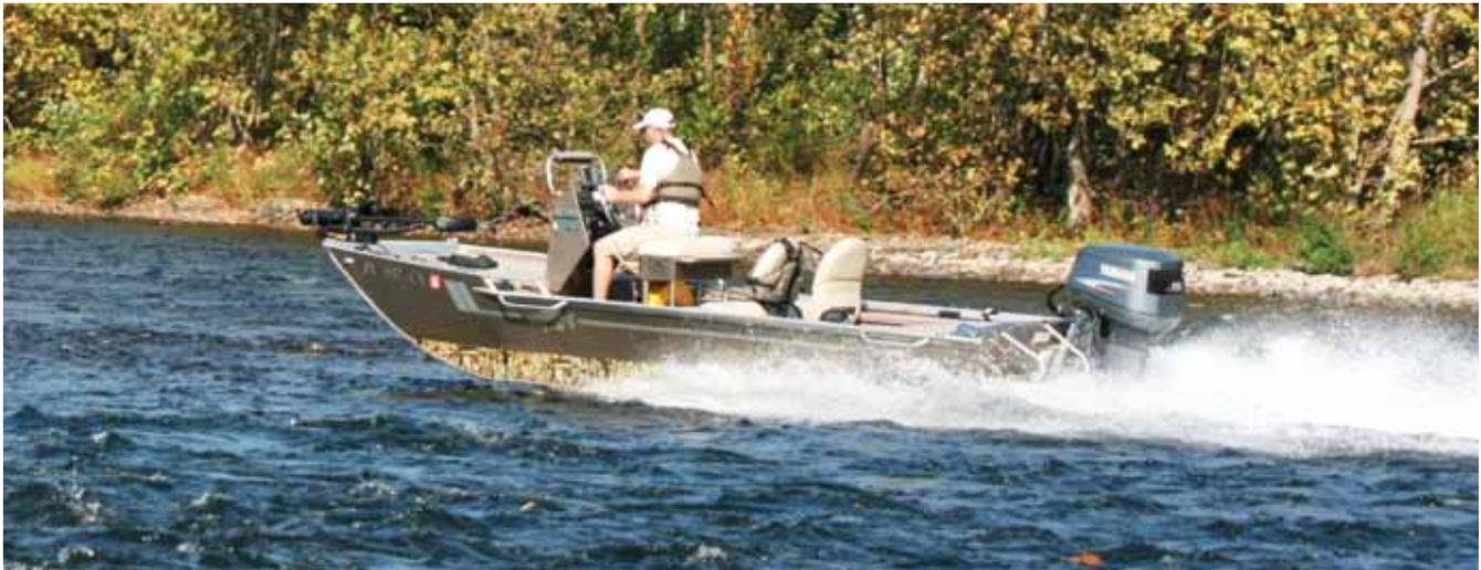
With an outboard jet drive, the water enters the bottom of the jet intake and is turned 180 degrees. It is expelled through the exhaust housing. The result is a 30% loss in horsepower. With an inboard jet, the water enters the intake. After a short 28-degree ramp, the water passes directly through the impeller and out the exhaust housing. The inboard jet pump does not have to redirect the water giving it a significant performance edge to an outboard jet.
