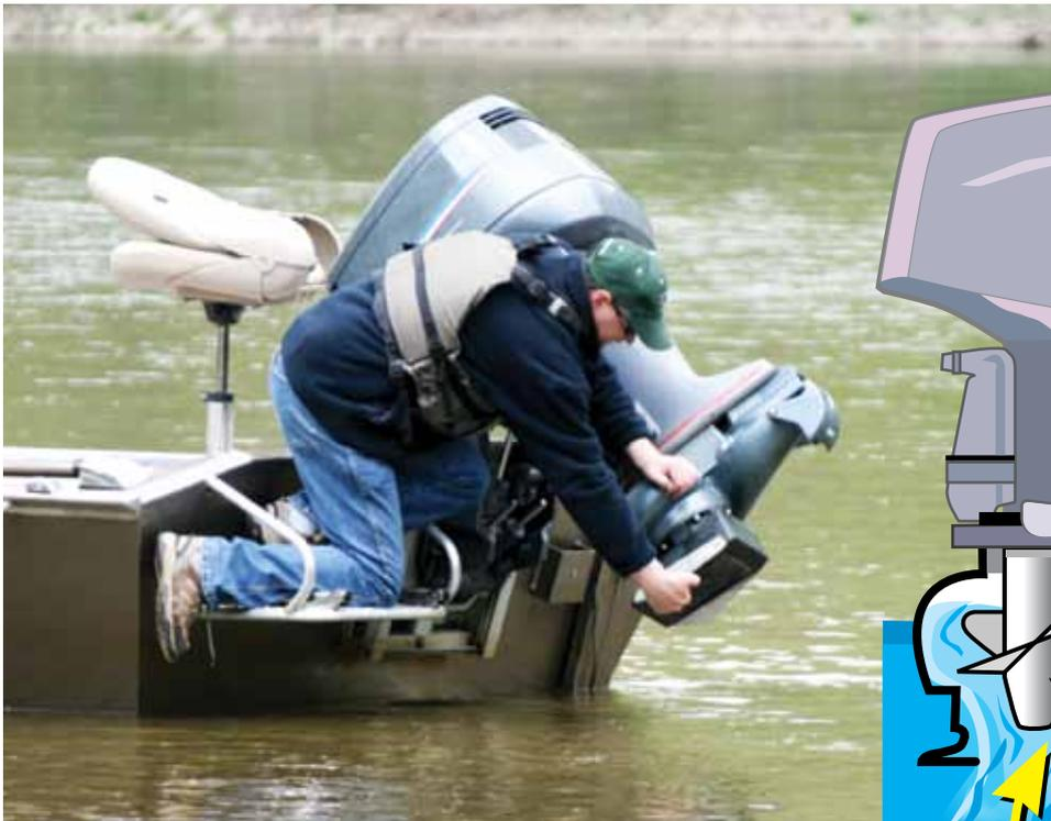
*With an outboard jet drive, the water enters the bottom of the jet intake and is turned 180 degrees. It is expelled through the exhaust housing.*
