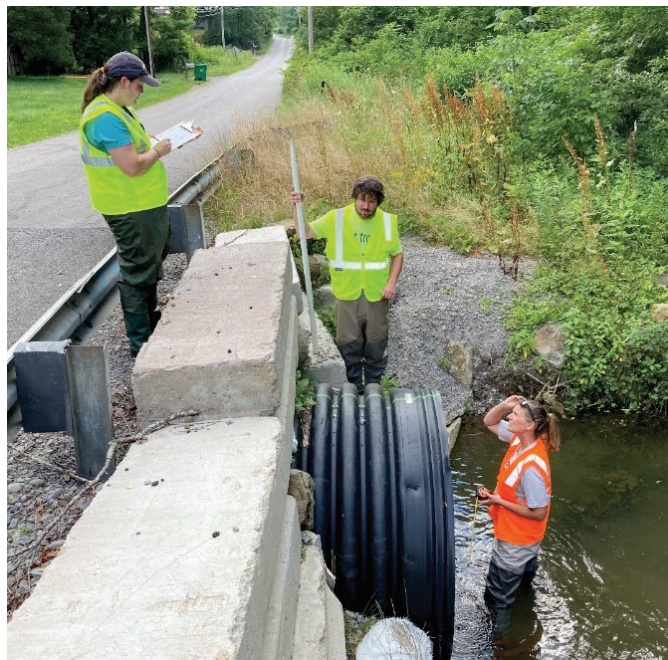
PFBC staff train faculty and staff from Allegheny and Thiel colleges on how to assess road-stream crossings.
