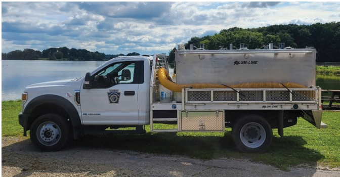
One of the new stocking trucks with insulated aluminum tanks.
